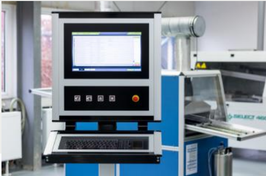
HMI system with capacitive operating elements and surfaces made of glass
